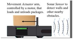
Figure 1: Sensors and Actuators for a Warehouse Robotic Package Handler.
